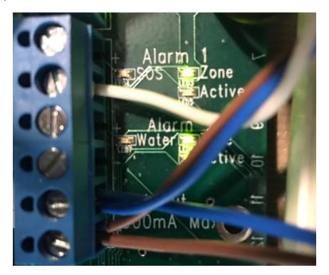
With a Nautic Alert beam sensor, setup is a breeze and does not require any complex calibrations. In the configuration shown above, when the beam sensor emitter and receiver are facing one another, the zone active light is not illuminated. A loss of the beam pattern from the emitter will cause a zone activation.
